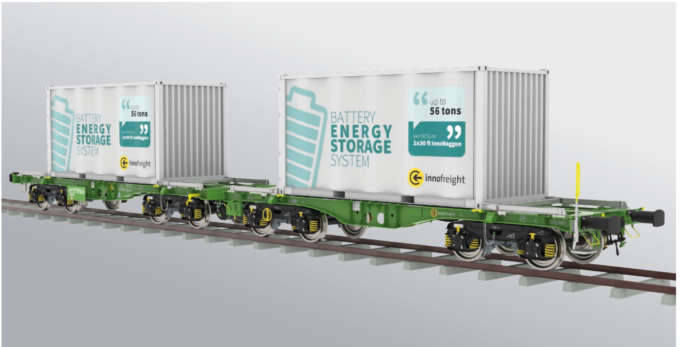
2x30 ft InnoWaggon with HeavyDutyLoading System and two 20-foot-long BESS modules
