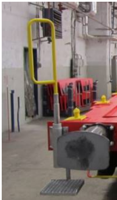
Figure 6 Foldable handle – set up
