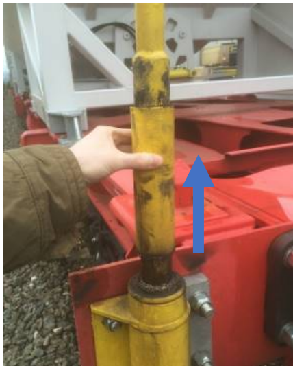
Figure 7 Foldable handle – lifting the sleeve
