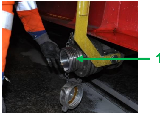
Figure 151: Type G, Before emptying D.1.2.
