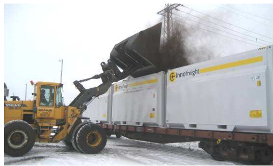
In the station: loading of biomass with wheel loader (e.g. in terminals)
