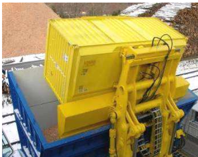
Unloading technique: stationary or mobile unloading of the container with and without HardTop.
