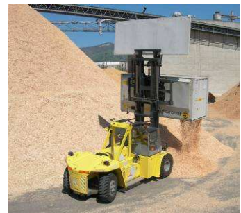
Unloading technique: stationary or mobile unloading of the container with and without HardTop.
