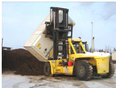
Unloading technique: stationary or mobile unloading of the container with and without HardTop.
